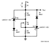
FIGURE 9. Bidirectional Adjustable Clamp ±2.4V to ±6V
