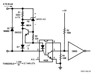
FIGURE 12. Precision Floating Current Detector
