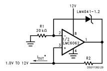
FIGURE 13. Precision 1  $\mu A$  to 1 mA Current Sources
