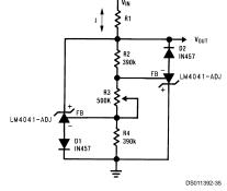
FIGURE 8. Bidirectional Adjustable Clamp ±18V to ±2.4V
