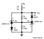
FIGURE 7. Bidirectional Clamp ±2.4V
