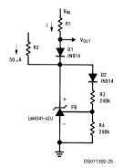
FIGURE 6. Fast Positive Clamp 2.4V + V<sub>D1</sub>
