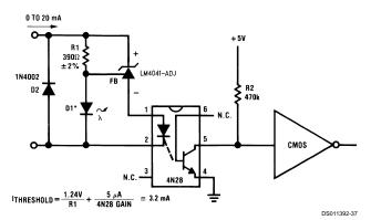
FIGURE 10. Simple Floating Current Detector
